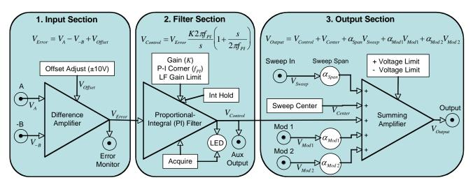
Figure 7: Schematic of LB1005 Signal Architecture
