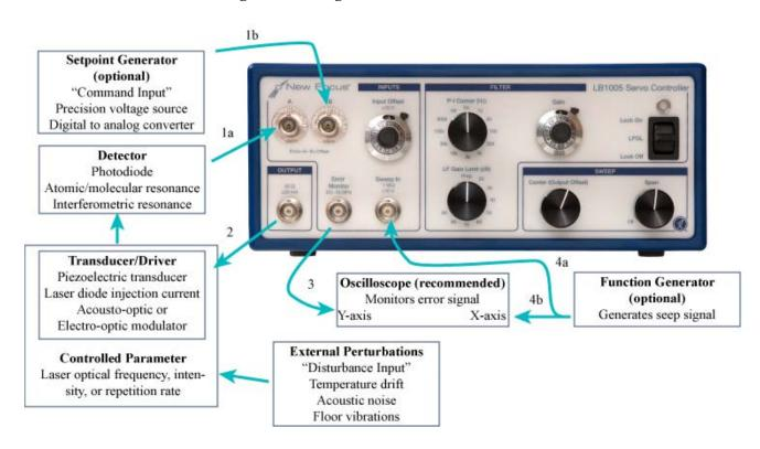
Figure 3: Typical signal connections for LB1005
