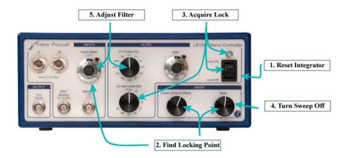
Figure 5: Typical Operation of Controls
