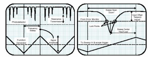
Figure 4: Typical oscilloscope signals are shown for locking to the side of an optical resonance. The dashed horizontal lines indicate ground for denoted signals. a) A triangle
